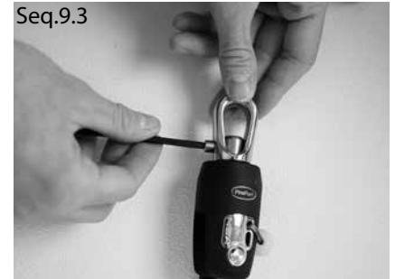
Seq.9.3 Monter l'oeil et serrer la vis Fit the eye and tighten the screw
