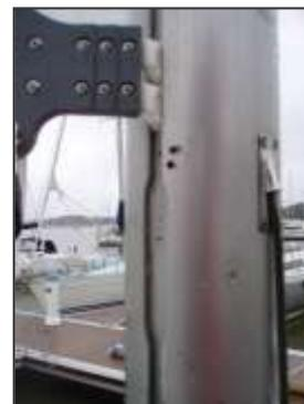
**III.5.B** – Cut carefully with cutter blade the lower part from the luff triangle (15) to the “Y” value from the upper part (Picture A). Cut up the luff line 50mm (1 31/32”) shorter than the cut (Picture B and C).
